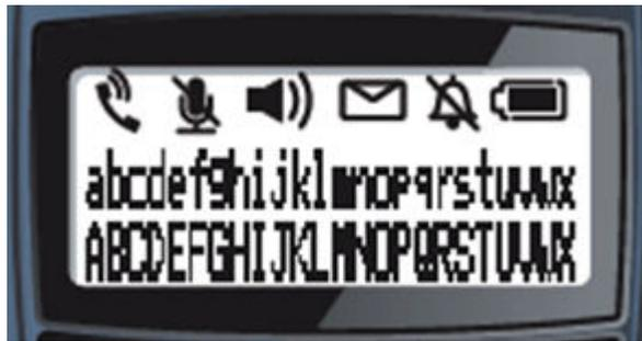
The handset LCD consists of three rows. The top row consists of six icons while the remaining two rows consist of 24 alphanumeric characters.
