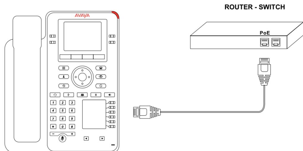
2. If your router does not have PoE port available, connect the J159 ethernet port to the available port on your router. Connect the power adapter to the J159. The device bootup will start.
